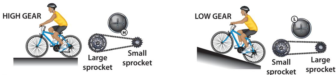
**Shifting Gears** A car's transmission works just like the gears in a bicycle. High gear combines the larger crank sprocket with the smallest sprocket at the rear wheel. *What combination of sprockets does low gear use?*
